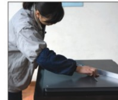
Flatness Test 平整度测试
