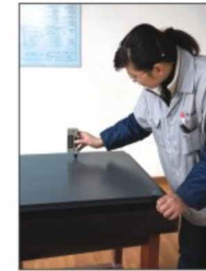
Coating Thickness Test 喷粉厚度测试
